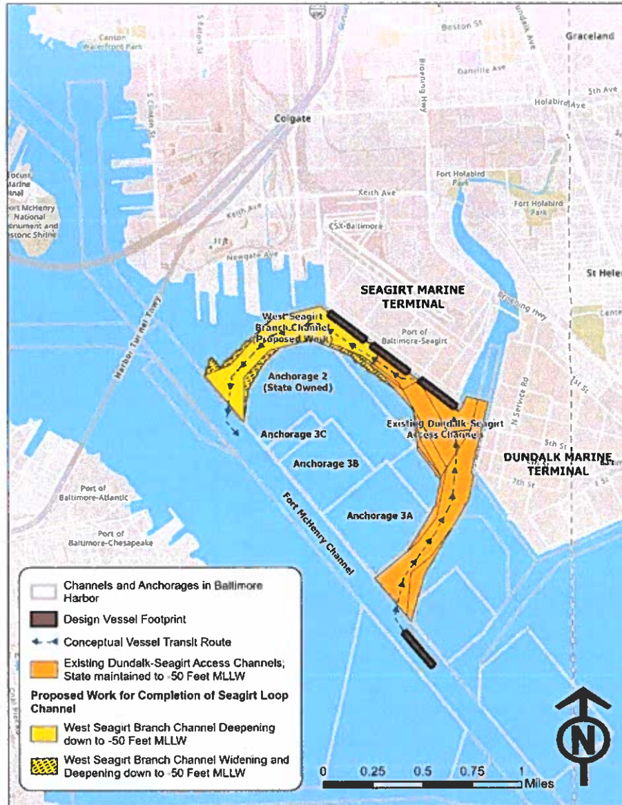
Proposed Project Alternative – Deepening and Widening of the West Seagirt Branch Channel (yellow).
